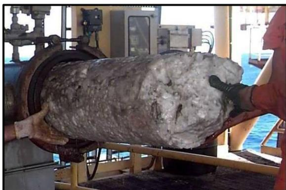
Figure 1(b). A large gas hydrate plug formed in a subsea hydrocarbon pipeline (Picture from Petrobras - Brazil).
