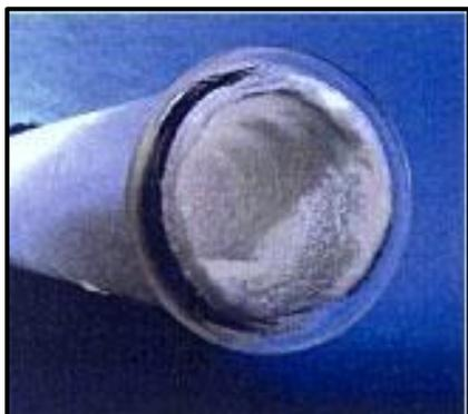
Figure 1(a). Adhered Hydrate on internal walls on gas pipelines (Picture from Repsol YPF)
